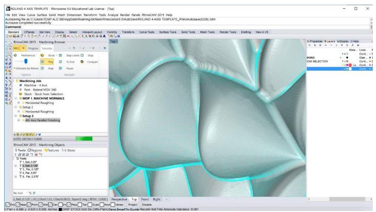
Zoom in and check out your toolpaths. These types of paths would be impossible to realize without the simultaneous movement of the 4th axis component.
