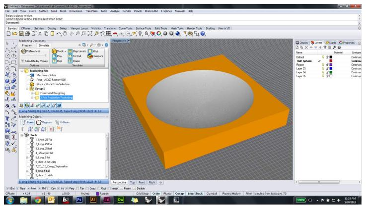
Under the Simulate tab run the simulation to see the final surface with the Projection Pocketing. Check to make sure there are no collisions or errors in the milling paths.
