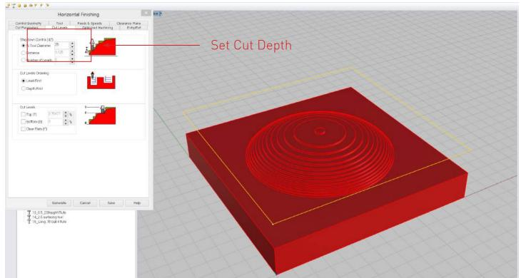
Under Cut Levels, set the cut depth to match the vertical spacing between the contours in your model. In this example, each contour is 1/8", so the cut level is 25% of the tool diameter. 25% of the 1/2" endmill = 1/8", so we will catch every contour in our model. If the cut level does not match your contour heights, the software may skip levels.
