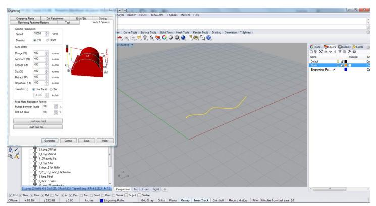
The feeds and speeds will be determined by the material being milled and the type of endmill selected. Please see the feeds and speeds section and consult the Fab Lab.
