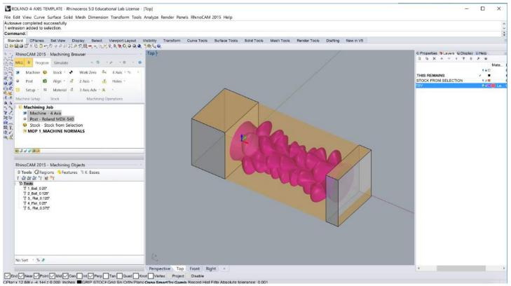
Position your desired geometry within the millable region, centered on the x axis. Your geometry should be fully encased within your stock material, and attach to the leftover fixturing material at either end. Geometry cannot simply float within the bounding volume
