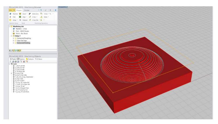
Once all the parameters have been set up press generate to create the milling paths.
