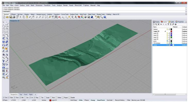
In the sample above a terrain file has been imported into Rhino, the mesh was generated from contour data. The surface will be placed in a piece of stock that will match the physical stock to be milled. Both meshes and nurbs surfaces can be used for 3d milling.
