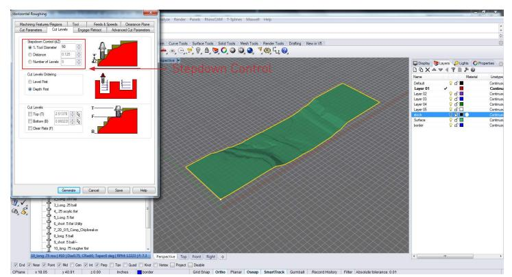
Under Cut Levels the stepdown control can be set, either the distance or the tool diameter can be set to determine the levels for the Horizontal Roughing.
