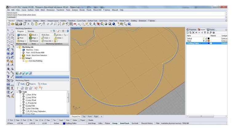
Once generated the profiling path will appear in the Program Tab view, the light blue lines are the bridges and the dark blue is the profile tooling path.
