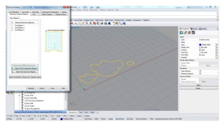
For multiple profiles, select all the drive regions as long as the cutting operation performed remains the same. Under the Sort tab select minimum sorting distance.
