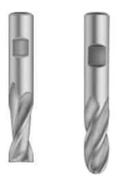
End Mills come in different lengths and diameters, the daniels tool library (covered previously in how to load the tool library) has a range of end mills from 1/4" to 3/4" in flat end mills and ball end mills. The end mills have a overall length, cutting depth and both shank diameter and mill diameter.
