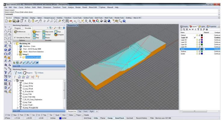
Run the simulation under the simulate tab to make sre there are no collisions or errors in the tooling path setup.
