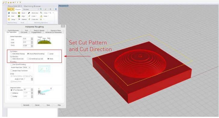
Under the Cut Parameters set the Cut Pattern to Part Offset and the Cut Direction to mixed. The tool diameter is set to 25% in this example, for less dense material it can be set higher to speed up the Roughing Pass.
