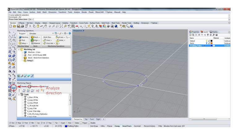
The direction of the curve can be flipped while in the Analyze direction command. These curvature directions will be important in assigning 2D milling operations as the line/ curve direction will dictate the cutting direction in your milling operations.
