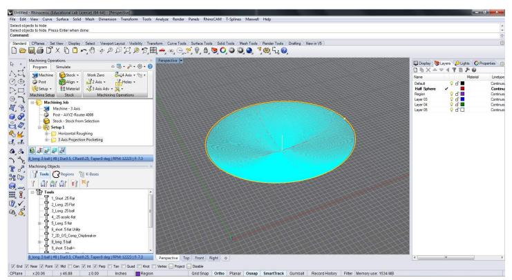
Once all the parameters have been setup press generate to create the tooling paths, parameters can be re-adjusted if tighter / looser milling paths are required.
