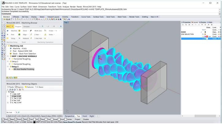
Generate this operation to view its toolpaths. Notice how they stop short of the vertical faces of our fixturing geometry.
