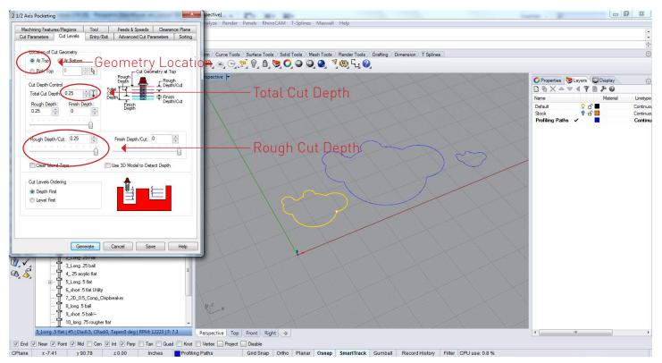
Under Cut Levels the depth and step down of the cut is defined, chose the geometry location, the curves in the example are located at he top, the rough cut depth is set to match the total depth as the cut is only .25" if great the rough cut depth is set to step down, this is done through the slider to set the steps to the total cut depth
