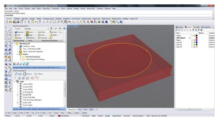
For the pocket projection we will start off with a horizontal roughing pass to clear out the material from the inside of the half sphere before the finishing pass with the projection pocketing.
