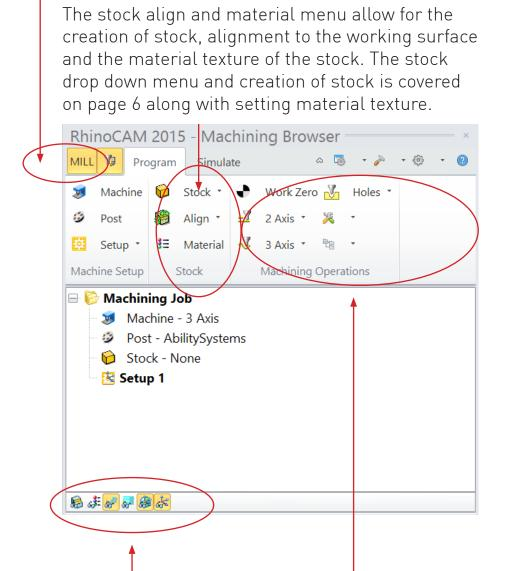
The display buttons are located in the bottom left of the machining operations menu. From left to right they display the stock visibility, material texture visibility, toolpath visibility, toolpath level visibility and Machine CSYS visibility.
