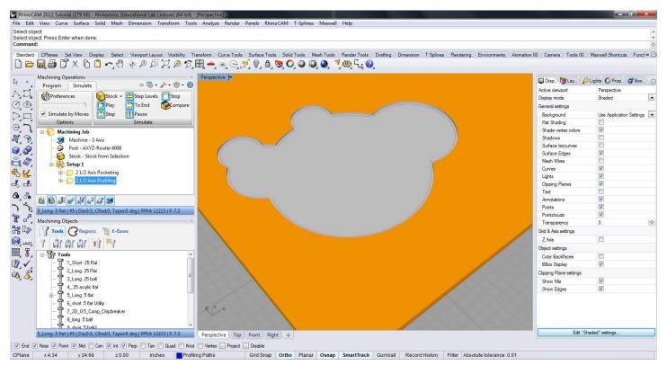
Once the profiling pass is simulated you will see a small stepover from the pocketing pass to the profiling pass, the new cut profile is tight to the original curvature.
