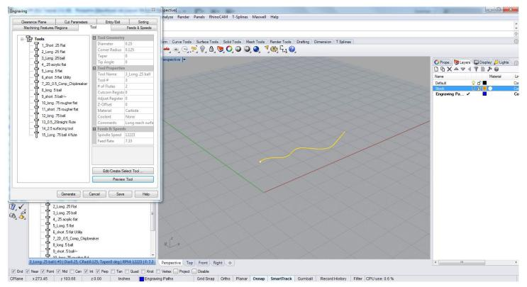
The endmill diameter selected will determine the width of the engraving line, as the endmill center point follows the selected engraving line the tooling path with be the endmill diameter from the center of the line.
