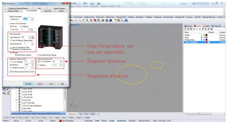
Once the regions have been set, set the chosen endmill and the feeds and speeds required for the material to be milled. Under the Cut Parameters chose the location of the geometry, next set the hole depth and check "Use Arc Diameter as Hole Diameter for all selected arcs". Chose the stepdown distance and stepover distance based on the endmill chosen and the material being milled.
