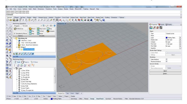
The tooling paths generated will be sequential from the start regions selected from the sort tab, this will speed up operations when multiple profile cuts are performed.
