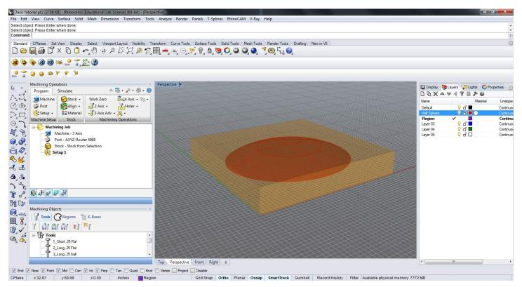
For Spiral Machining the same process will be repeated from the projection pocketing example. Begin with placing the poly object in the stock and then use Horizontal Roughing to remove the material before the final milling pass with Spiral Machining.
