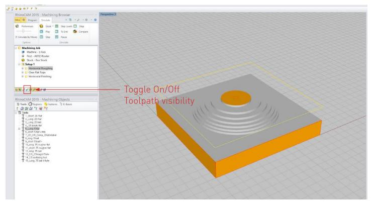
Toggle off the tooling paths to view the Horizontal Roughing path surface.
