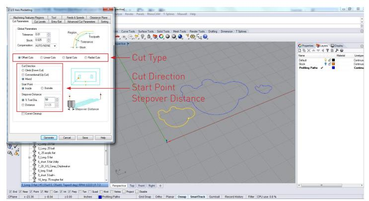
Under Cut Parameters the pocket can be cut using either Offset, Linear, Spiral or Radial cuts. The choice of operation will be dependent of the geometry to be pocketed, for the curvature shown the offset cut will be used starting from the inside to perifery of the geometry, The stepover is set to 50%.
