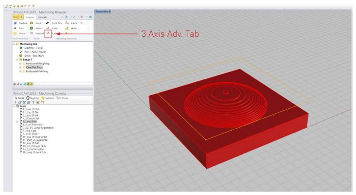
Under the 3 Axis Adv select the Clear Flats tab. This operation is useful if the horizontal distance between your contours is larger than the diameter of the endmill, and will clear excess material before your final finishing pass.
