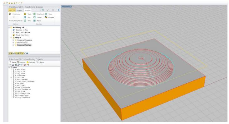
Under the Simulate Tab run the tool path simulation to make sure there are no collisions and that the tooling paths generated are the desired ones.
