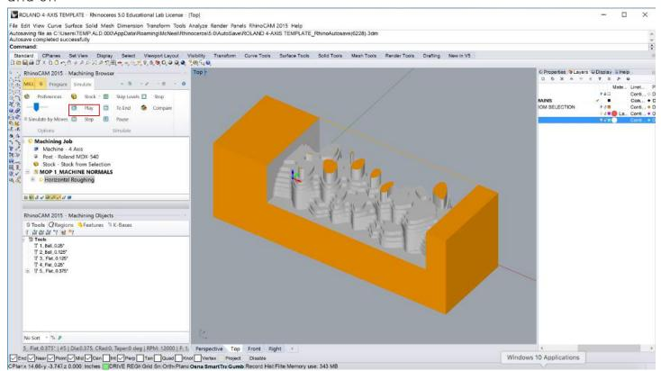
Highlight the Horizontal Roughing operation and click 'play' in the Simulations tab. Toggling the toolpath visibility on and off will show you the results of our roughing operations so far. Notice that we have only gone to 0, and the bottom side remains.
