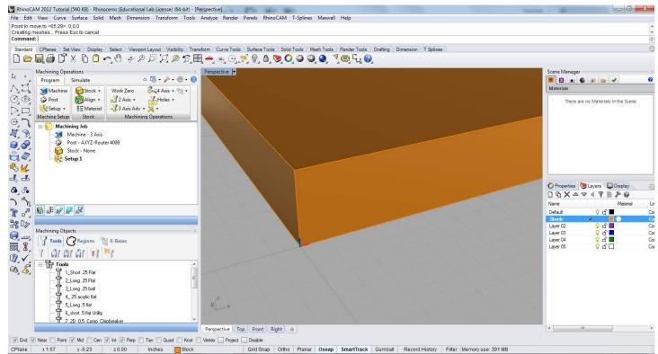
Move the stock to the origin in rhino (0,0,0) this corresponds to the origin of the CNC. The Red, Green and Blue arrows indicate the X,Y and Z direction of the CNC bed.
