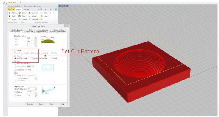
Under Cut Parameters The Cut Direction is set to Climb and the Stepover Control is set to 25%.
