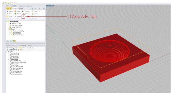
Under the 3 Axis Adv select the Horizontal Finishing tab. This operation will detect the vertical faces in your model and treat them as if they were profile curves. This should give you a nice clean finished contour edge.
