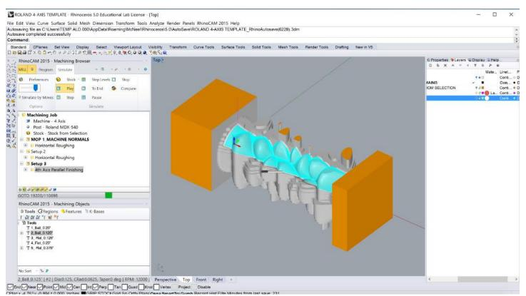
Simulate this operation to view your results. Again, in reality the part spins, not the approach of the endmill. It's just a RhinoCAM simulation quirk.
