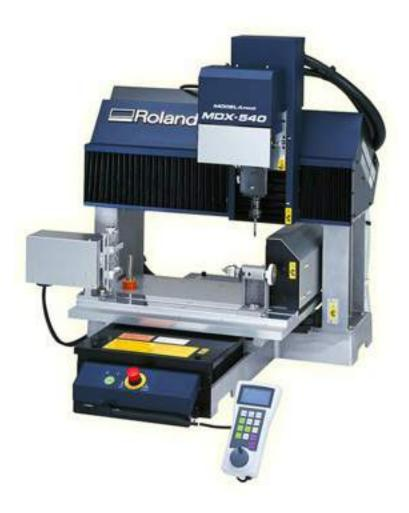
The Roland MDX 540 is a small scale CNC 'lathe' that allows for the fabrication of highly detailed components and geometries that would be impossible to achieve in 3-axis milling. A rotary axis allows the stock material to turn slowly during milling, allowing the endmill to gain acess to areas that would be considered 'undercut' on a 3 axis machine.
