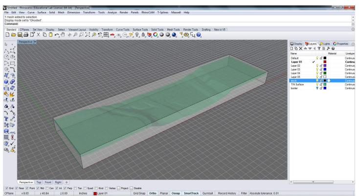
Create a stock to match the physical milling stock, place the terrain within the stock, try to allow as little as possible distance between the top of the stock and the terrain. This will allow for reduced milling time. The deep the terrain is inset into the stock the more material there is to remove for the finished topography.
