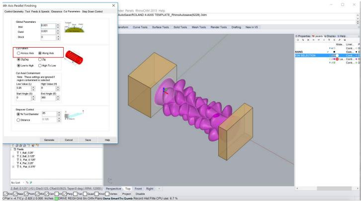
In the cut parameters tab, we need to define a few variables. First, whether we want to cut along the axis vs across. This is a choice you can make depending on your geometry, for now the along axis works fine.
