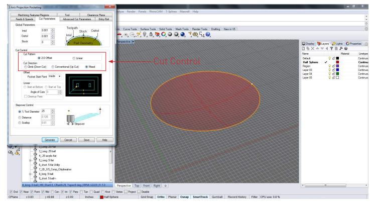
Under Cutting Parameters set the cut direction to mixed, the cut control is set to 2D Offset, linear can be selected depending on the resultant tooling paths desired. The stepover is set to 25% for a smoother final pass.
