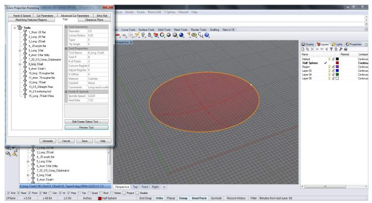
Under Tool select a ball endmill to create a smoother finishing pass, in the example the Daniels long 1/2'' ball endmill is selected.
