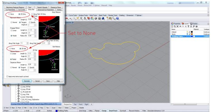
Under the exit / entry tab set the entry and exit motions to none, the 2d exit will create a turn out cut that can come close to other profiles if there are tightly nested.
