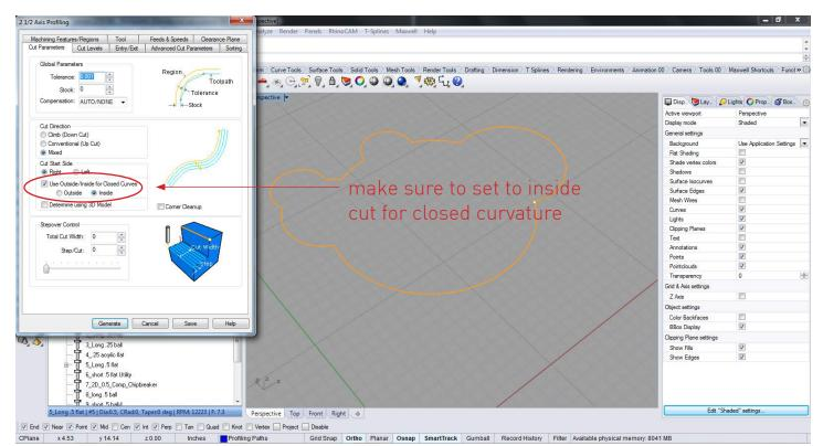
Select the same curvature used for the pocketing pass, in Cut parameters make sure the use outside/inside curves is selected and set to inside. set the depth the same as the pocketing pass.
