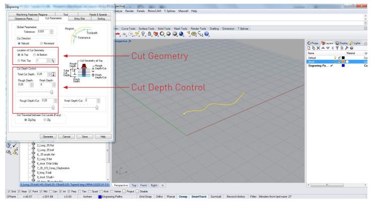
Under the Cut Parameters tab, the cutting direction, depth and geometry location is chosen. The geometry currently in the example is located at the top, the total cut depth is 1/4", this is done in one pass, for deep milling the depth can be done in multiple passes by setting the rough cutting depth and the finish cut depth.
