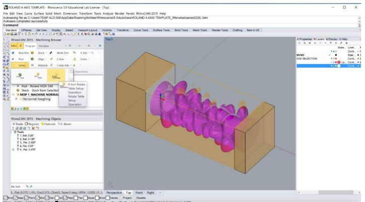
The Machine Operation Set (CSYS Setup) we used for the first roughing pass uses the Rhino axis' to determine part orientation, ie. Rhino Z is 'up'. This is the default setup type. Now, we need a Machine Operation Set that will change the orientation by 180 degrees in order to mill from the bottom. Click setup, then Rotate Table
