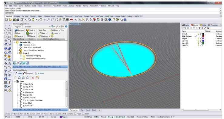
Once all the settings have been completed press generate to view the tooling paths created by the input parameters.
