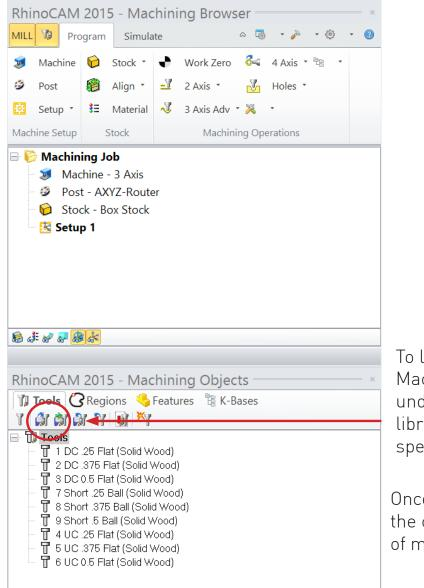
To load the tool library go to the Machining Objects Menu while under the tools tab click the load tool library button. Only load the tools specific to your material.
