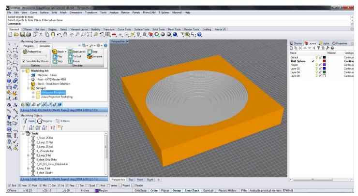
Go to the Simulate Tab and run the simulation to make sure there are no collisions or errors in the tooling path setup.
