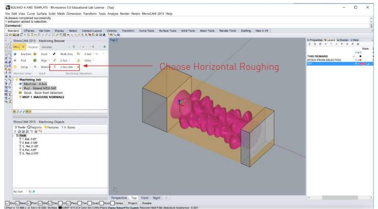
We will rely on 3 axis milling operations to perform a roughing pass from both top and bottom in order to clear out stock material before finishing passes can be run. Select 3 Axis Adv. operations from the Machining Browser, and choose Horizontal Roughing.
