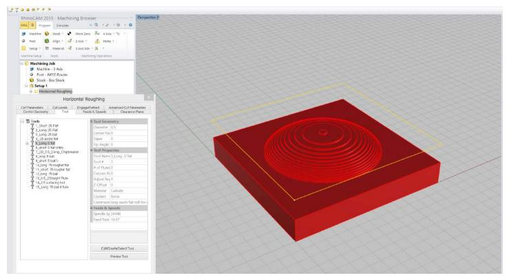
Under Tool for the Roughing pass select the .5" long Flat endmill.
