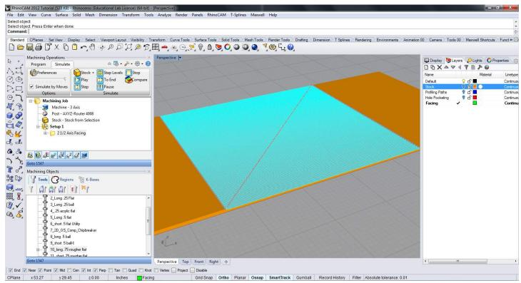
Once the tooling paths have been generated run the simultaion under the simulate tab.
