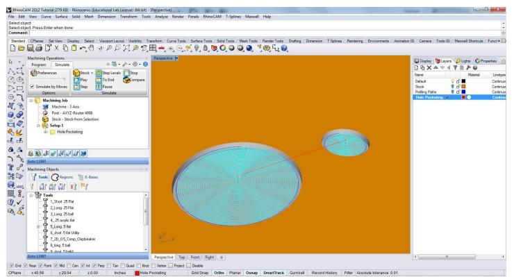
Run the simulation to see the milling paths in process, always run the simulation to make sure there are no errors or collisions with the collet or head of the CNC.
