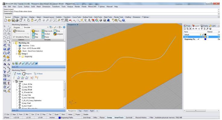
Once the milling paths have been generated select the simulate tab and run the engraving paths to see the toolpath result.
