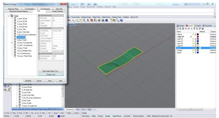
Under the Tool selection tab, select the tool used for the final finished surface mill. For the topography a .5 ball endmill is selected to give a smooth finish with a slight scallop from the stepover of the ball endmill.
