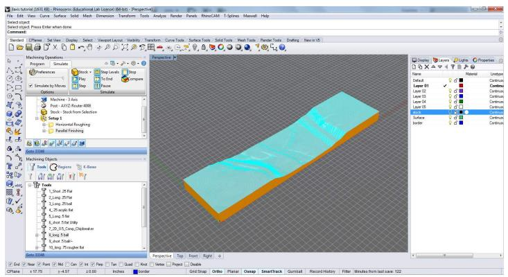
Under the simulate tab run the simulation to ensure that there are no errors or collisions in the tooling paths.
