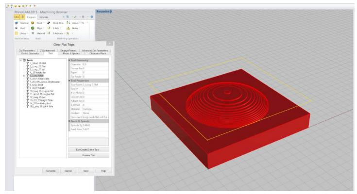
Under the Tool tab select the endmill for the finished surface, the long .5" flat is used in this example.
