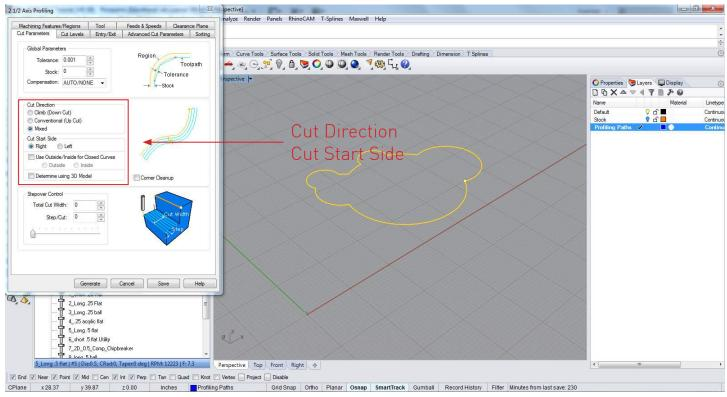
In the Cut Parameters tab the cut direction can be changed and for closed curvature either the inside or the outside of a closed curve can be chosen to cut. A offset of the profile can be setup with Stepover Control, the cut width and the step over to the desired width can be set up here. As a general rule never cut deeper or step over more then half of the diameter of the chosen endmill, for denser materials this should decrease.
