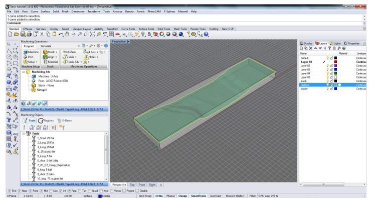
Create a bounding region around the terrain to be milled, this can be a flat region or following the terrain edge. This region will assign the surface to be milled.
