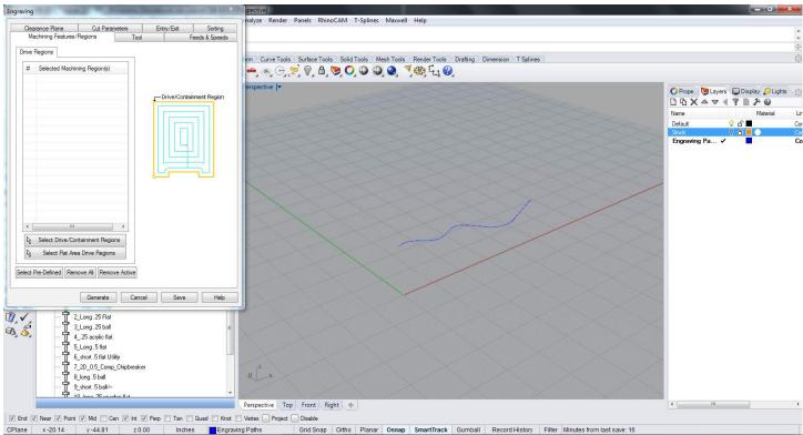
Select Engraving from the 2D milling operations tab, press select drive/containment region to select the engraving milling path(s) established.
