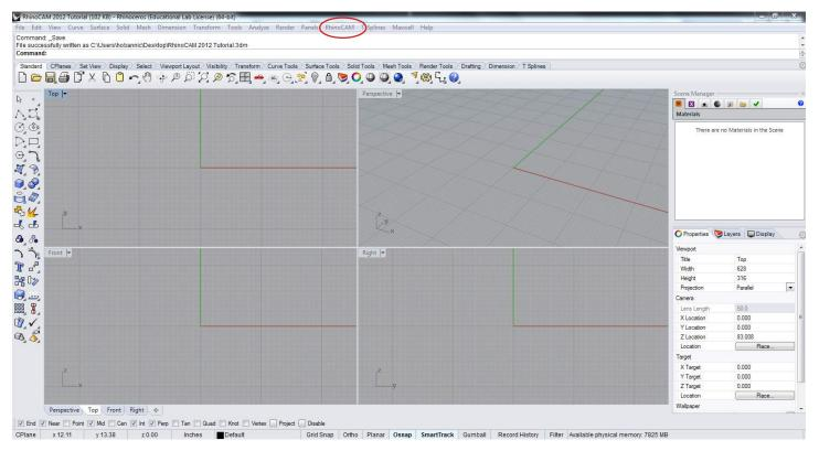
To operate RhinoCAM launch the Machining Operations Tab and the Machining Objects Tab. These can both be found in the RhinoCAM Drop down menu located along the top of the Rhino menu.
