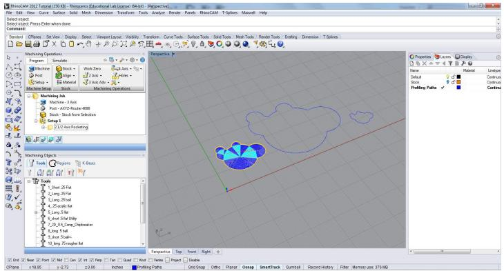
Once all the parameters have been set press generate, the tooling paths will appear in a offset orientation starting from the inside working outwards to the curvature.
