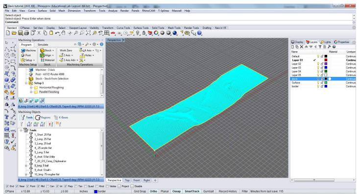
Once all the parameters have been set up press generate and the surface will be populated with milling paths following the finish surface of the topography.
