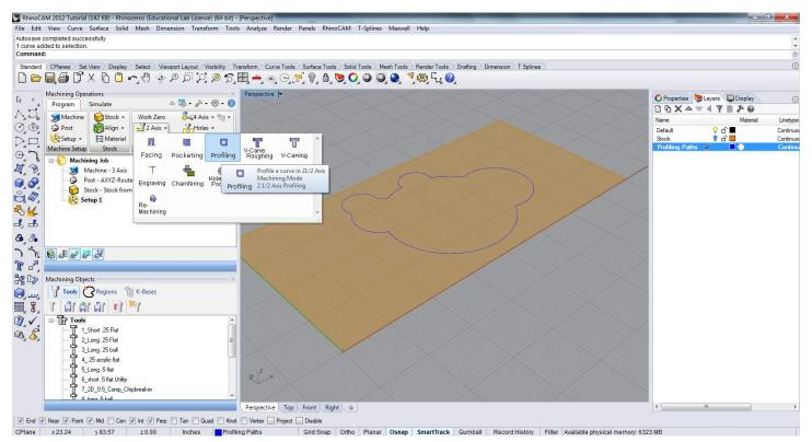
The Profiling tab is located under the 2 Axis machining functions in the program tab in RhinoCAM.
