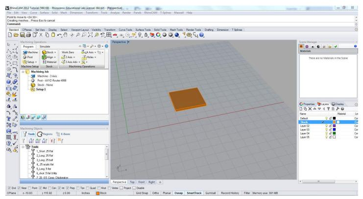
Create a stock layer, then create the stock size required to match the physical material stock. Create the stock in Rhino.
