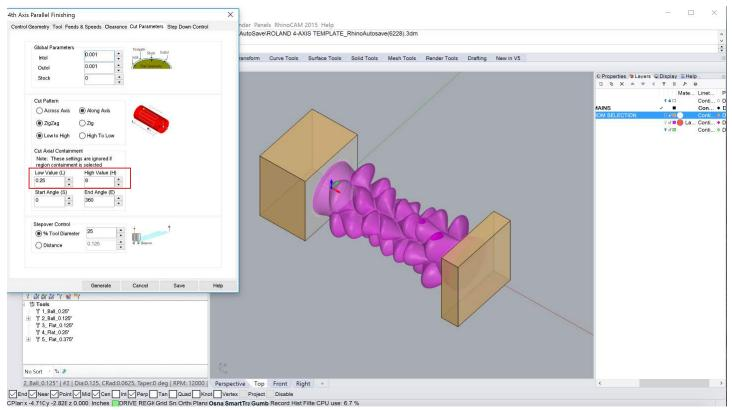
Next, we define axial containment. We want to keep the endmill off of those harsh vertical faces to reduce cutting strain, so we tell it to only cut along the x axis between 0.25" and 8" (our actual geometry runs 0" to 8.25"). The default 25% stepover is fine for now.
