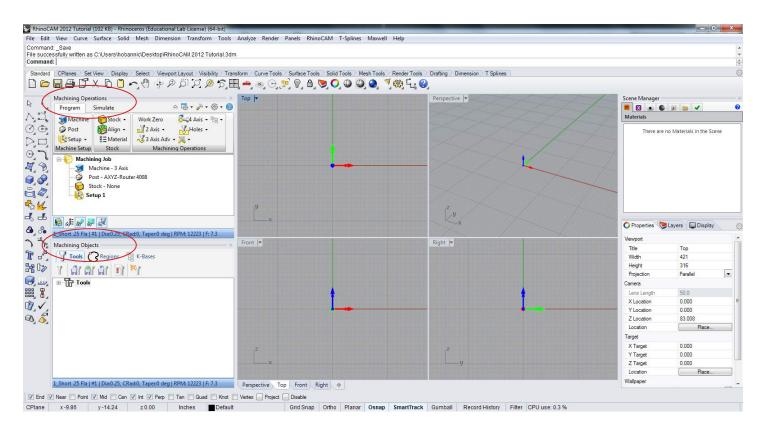
Once launched you can dock the two menus on the left side of the screen, both menus are necessary for setting up and running milling operations.
