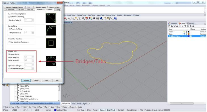
When cutting a profile out of a larger surrounding material the inner cut can lose suction to the CNC vacuum bed once cut. This can cause it to shift and bump into the endmill. To prevent this bridges can be created, these create small tabs that link the cut piece to the larger material. The height, length and number of bridges can be set. Once cut the bridges can be hand cut to release the profile from the material.
