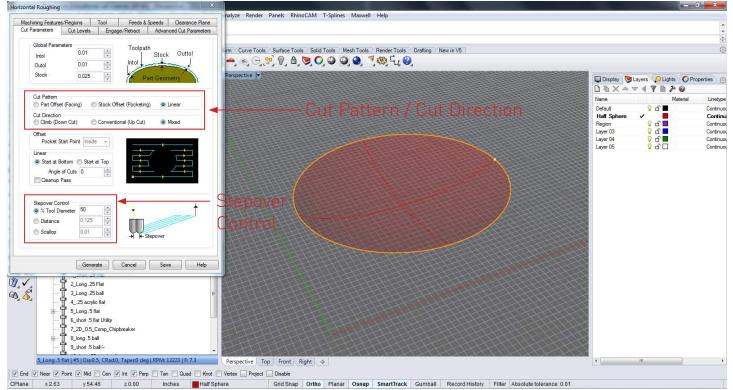
Under the Cut Parameters tab set the cut pattern to Linear and the cut direction to mixed, the stepover should be set accordingly to the material being milled.
