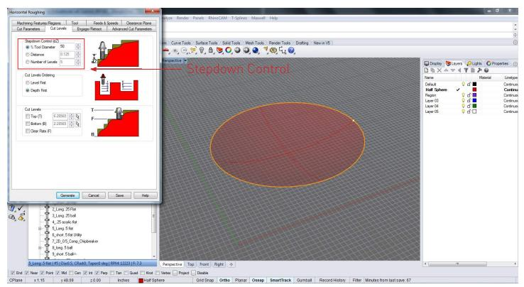
Under cut levels set the stepdown control to 50 percent of the tool diameter, this percentage can be higher for less dense material (ie foam).
