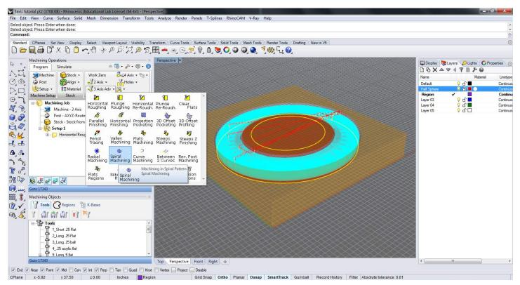
Under the 3 Axis Adv select the Spiral Machining tab.
