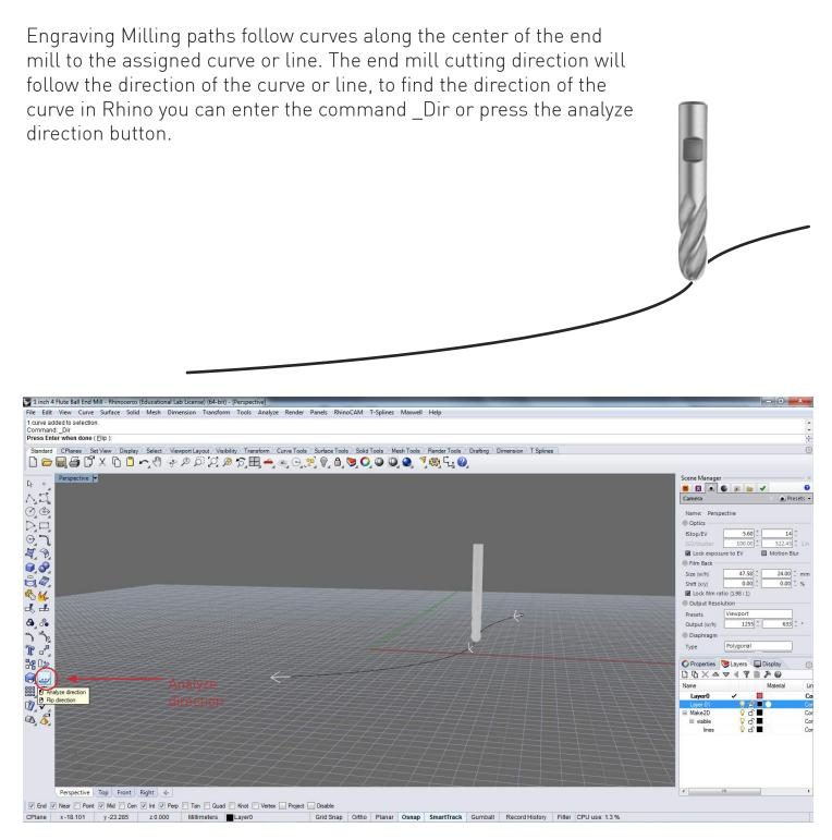
The direction of the curve can be flipped while in the Analyze direction command. These curvature directions will be important in assigning 2D milling operations as the line/ curve direction will dictate the cutting direction in your milling operations.
