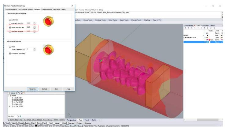
In the clearance plane tab, select stock max + 0.25". You should see that the clearance plane is represented by a cyclinder here rather than a flat plane.
