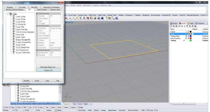
Select the endmill depending on the amount of material to be removed, for a larger area with geometry that is simple use a large endmill for faster facing. If the area is a smaller geometry select a smaller endmill to fit accordingly.
