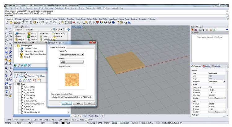
While in program tab when the material visibility is turned on the stock appears ghosted with assigned material type.
