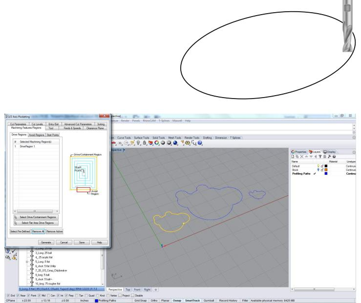
Using the same geometry as in the profiling path, select the desired drive/containment region. For a closed region the profiling path will be generated inside of the contained region
