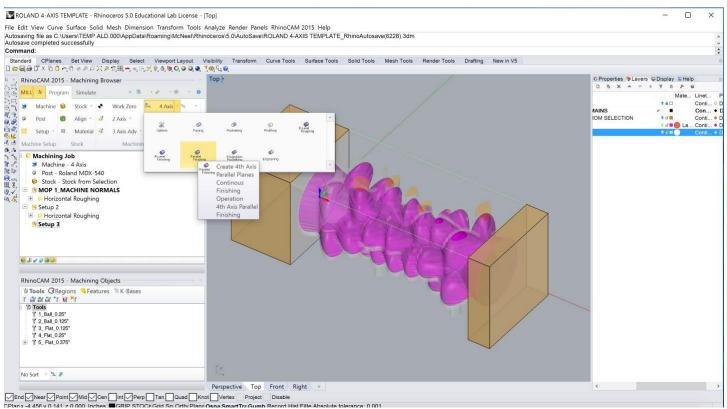
Click the 4 Axis tab and create a 4 Axis Parallel Finishing operation
