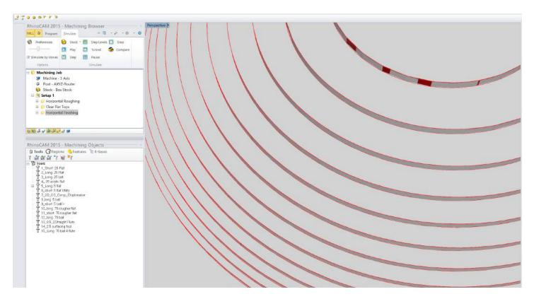
Once again you can turn off the tooling path visibility to see the simulated version of the final milled surface. You can see that the simulated results (grey) match our desired part (red).
