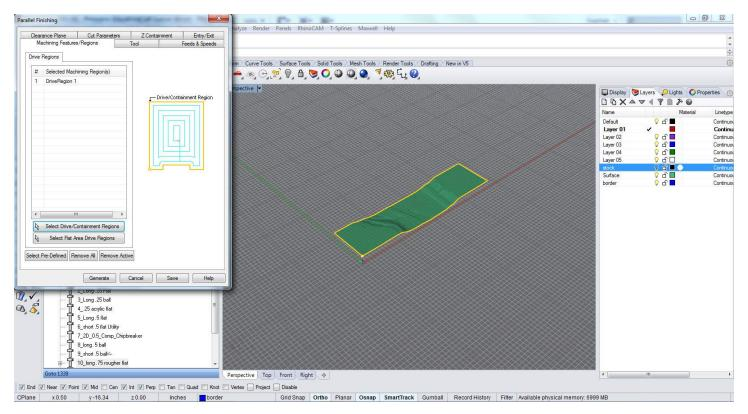
Select Parallel Finishing from the 3 Axis Adv drop down menu, select the drive region to be milled. This will be the same region used in the Horizontal Roughing pass.
