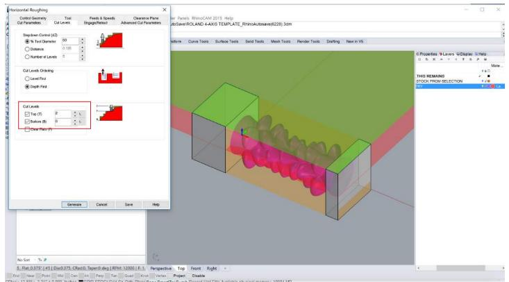
The automatic Clearance Plane, Advanced Cut Parameters, and Engage/Retract values can remain at their defaults. In the Cut Levels Tab, we need to set a manual Top and Bottom values to our cut. We are going to rough from both top and bottom to avoid undercuts, so setting the bottom to zero will have both operations meet in the middle.
