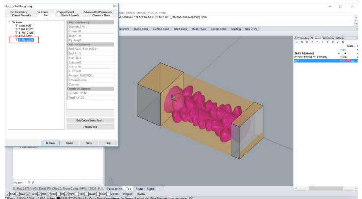
Select the tool you wish to use. In this case, using the largest tool at our disposal will speed up milling rates and allow us to remove more material more quickly.
