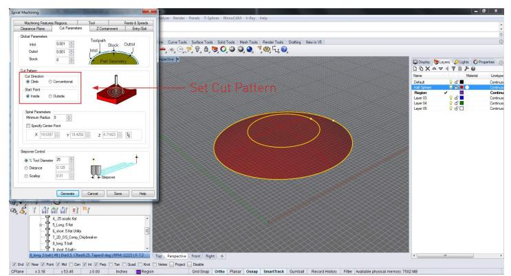
Under Cut Parameters The Cut Direction is set to Climb, the start point is set from the inside and the Stepover Control is set to 25%.
