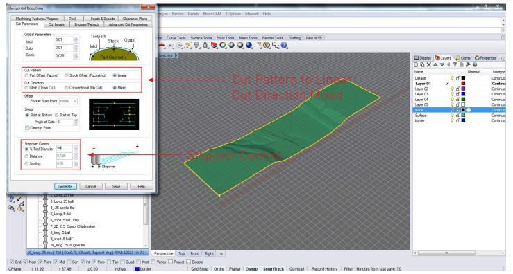
Under Cut Parameters set the cut pattern to linear and the cut direction to mixed for materials that cut direction isn't necessary (ie Foam). For stepover control set to half the endmill diameter for dense materials and for foam this can be increased to 75-100.
