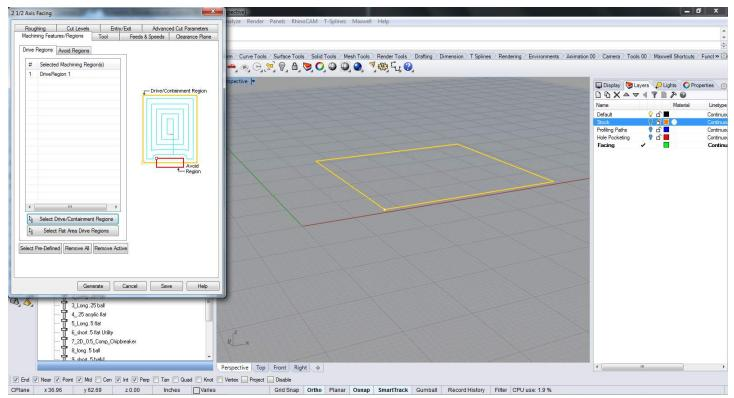
Select the 2 1/2 Axis Facing from the 2Axis drop down tab, select the region that is to be faced on the set up stock.
