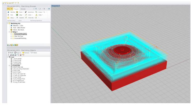
Once all the parameters have been set up press generate to create the milling paths.
