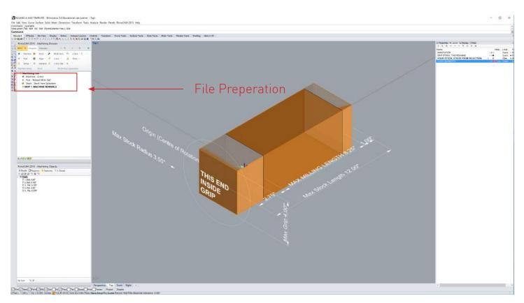
File Preparation : here, you will change the Machine from 3 axis to 4 axis, and the Post Processor to the Roland MDX 540. You will also set your 'stock from selection' as you would in any other 2 or 3 axis milling.
