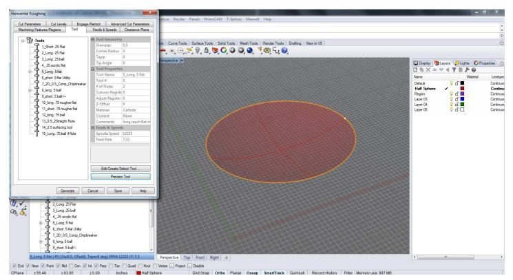
Select the proper endmill, dependent on the material being milled and the cutting depth required, in this example the long flat 1/2'' endmill is chosen from the Daniels tool library.
