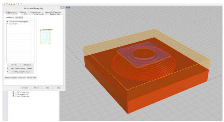
For the Horizontal Roughing create a drive region to contain the Horizontal Roughing pass. In this case the region is defined by the square profile of our stock material.
