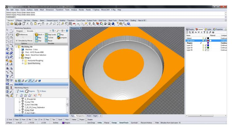
Once again you can turn off the tooling path visibility to see the simulated version of the final milled surface.
