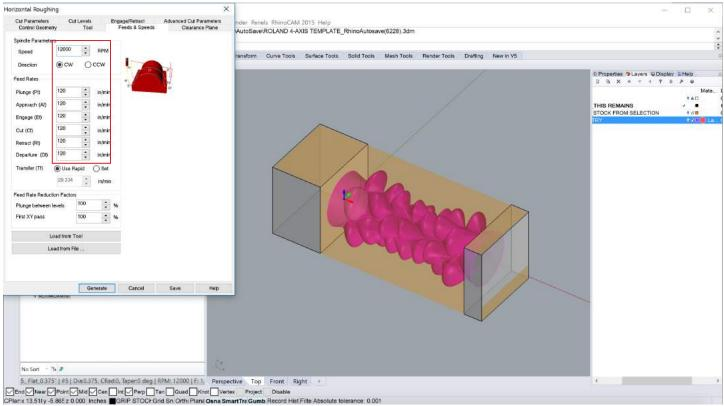
If you have loaded the Roland Tool Library correctly, these values should fill in automatically. A milling TA will review these with you prior to milling, as these values will change for each material. Note that the Roland MDX 540 has a maximum spindle RPM of 12 000 vs the 18 000 of our AXYZ 4008.
