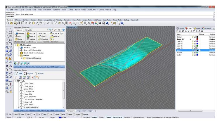
Press generate once all the setup has been completed, the tooling paths with levels will populate the surface.
