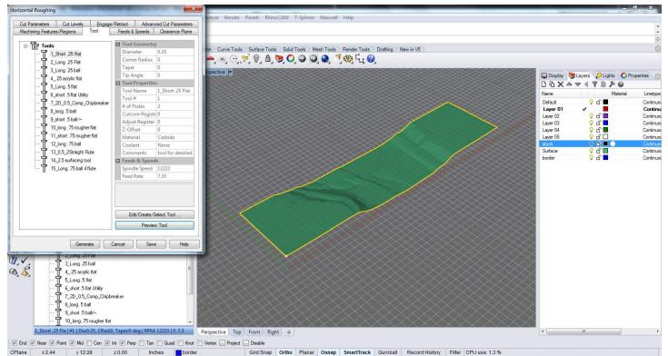
Select the endmill to be used for the roughing operation, typically a larger diameter flat endmill will be used to remove the material to approximate the rough surface.
