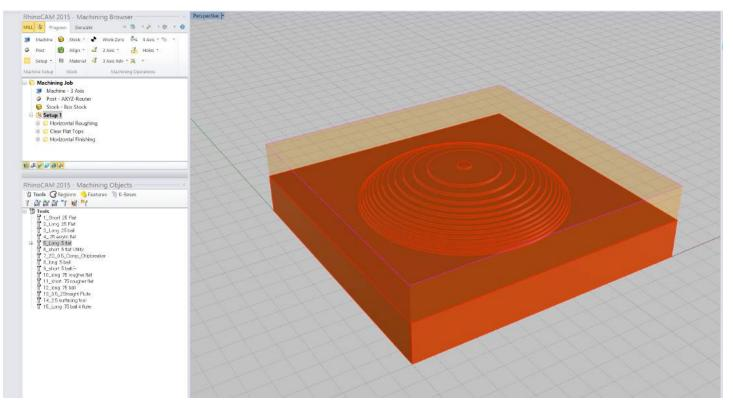
For Horizontal Finishing the same process will be repeated from the projection pocketing example. Begin with placing the poly object in the stock and then use Horizontal Roughing to remove the material before the next pass.
