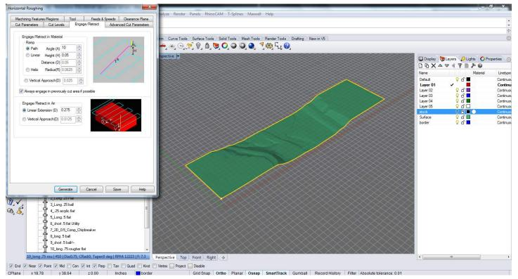
Under the engage/retract tab set engage/retract in material to path, the endmill will follow a path into the beginning tooling path.
