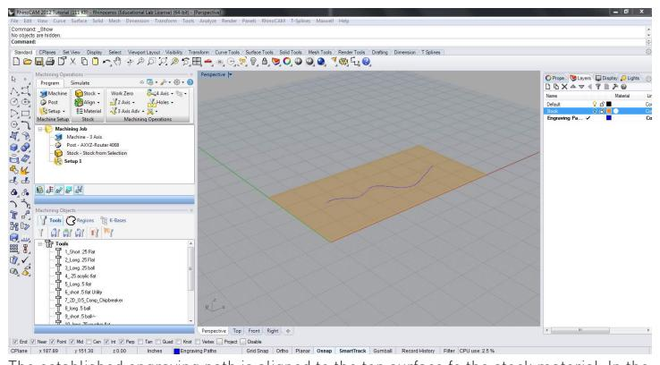
The established engraving path is aligned to the top surface fo the stock material. In the input parameters in the machining operations for engraving the cutting depth can be established.
