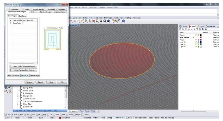
Select Horizontal roughing from the 3 axis adv drop down menu, select the drive region, this is the bounding region just created for the roughing pass.
