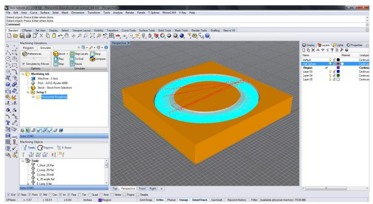
Under the Simulate tab run the simulation to check for any collisions with the head and make sure the milling paths are the desired ones.
