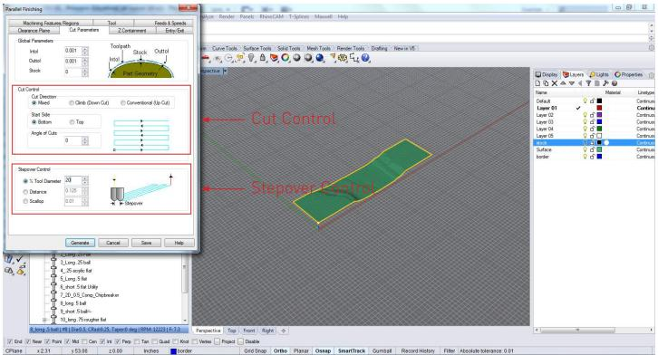
Under Cut Parameters set up the Cut Control, the direction is set to mixed and the angle is set to zero, if angled passes are desired set the angle of cuts to the chosen angle. The stepover control is set to 20%, the tighter the stepover the longer the milling time.
