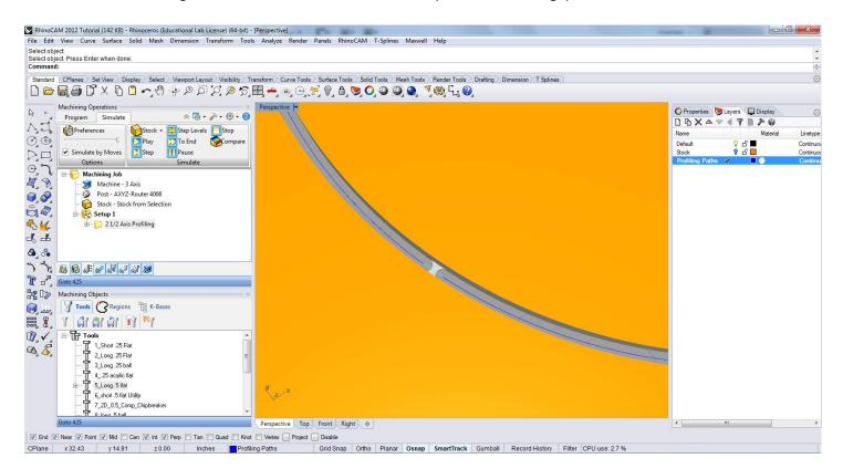
Under the Simulate tab once the simulation has been run the bridges are visible linking the profile cut back to the main sheet material.
